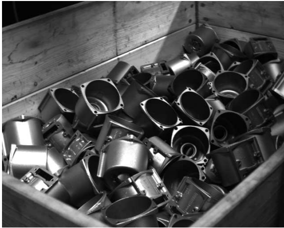
(a) A bin containing randomly organized stator housings.
