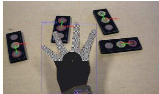
Figure 7. HMC input image with PHOs and a hand gesture showing segmentation results.
