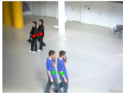
Figure 3.5: Tracking performed over two frames on two persons. The squares mark the median point at time t and the circle at time t+1 .
