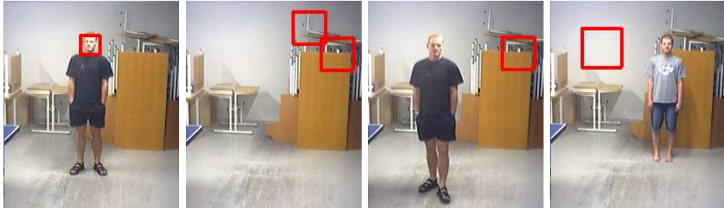
Figure 4.3: Examples of the OpenCV face detection, the first image show a correctly detected face while the second, third and fourth image show examples of false positives and negatives.
