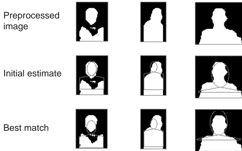
Figure 4.11: Three examples of the limitations of the head extraction. First column: nearly correct initial estimation, but mismatch due to segmentation errors. Second column: too small initial estimation (person seen from the side) causing erroneous head extraction. Third column: too large initial estimate, but since the head box is not allowed to exceed the original bounding box at the top of the person (not depicted), the head is extracted correct.
