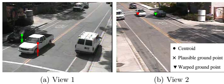
Fig. 6. The plausible ground point can be used to solve ambiguities in the overlap matrix. The many-to-many overlap occurs in this situation because the vehicle with red centroid in view 1 occludes the lower part of the vehicle with the green centroid.
