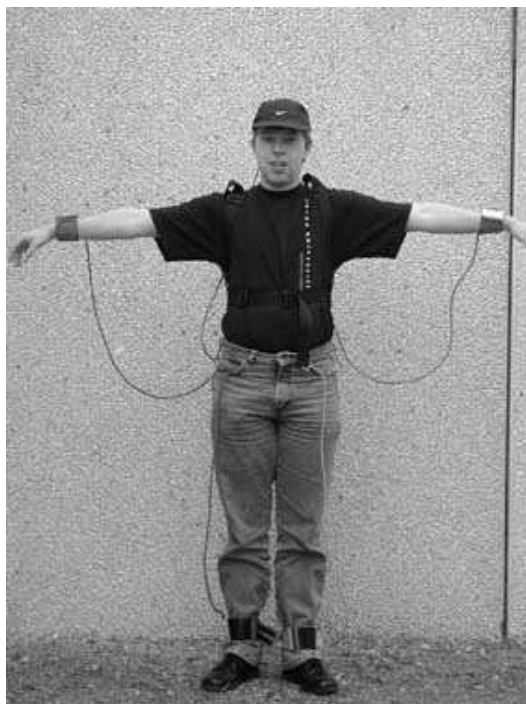
Figure 2.2: Electromagnetic devices mounted on a subject to capture his movements.
