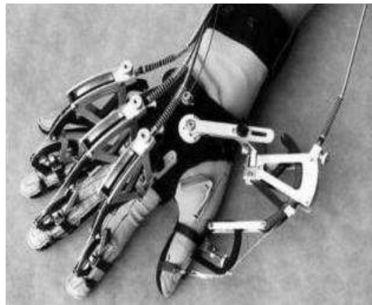
Figure 2.1: A mechanical glove for MoCap [3].
