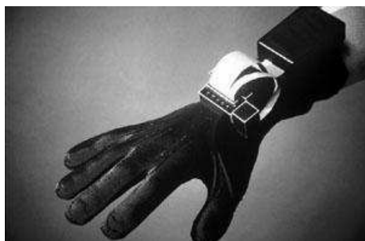
Figure 2.3: A fibre-optic glove (the 5th Glove) for MoCap [3].
