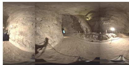
Figure 3: Longitude-latitude HDR environment map of chalk mine constructed from two hemispherical exposure sets. Due to slight lens vignetting the seams between the two hemispheres are visible as darkened vertical lines in the long-lat mapping. Tripod and photographer shadow artifacts are also visible. Such artifacts do not influence virtual object rendering noticeably. The dynamic range between the lamp and the floor is approximately 10000:1.
